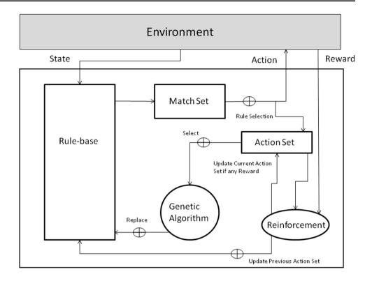
time step a match set is created. A system prediction is then formed for each action in [M] according to a fitness-weighted average of the predictions of rules in each [A]. The system action is then selected either deterministically or randomly (usually 0.5 probability per trial). If [M] is empty covering is used.
