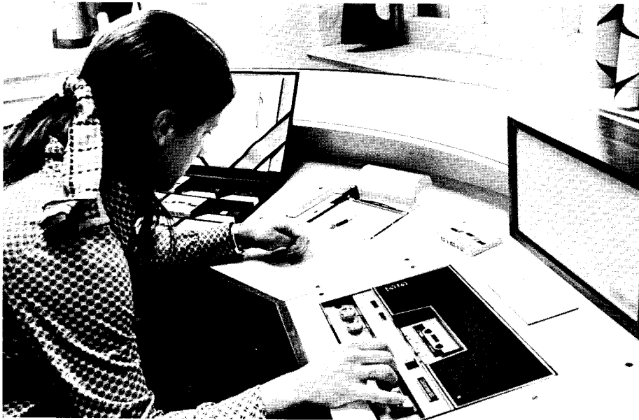
The console used by students in the experiment, with cassette deck, speaker, Electrowriter, and an album containing
